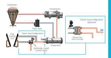
1 Mechanical Cooling Mode When it's too warm to use ambient air for cooling, the YVFA performs as a standard chiller. The automatic flow-control valve in the open-loop configuration bypasses the free-cooling coils to reduce pump energy. When either cooling load or ambient temperature are less than full design condition, the variable-speed screw compressors and condenser fans modulate to optimize energy use. In a closed-loop configuration, the free-cooling coils are also bypassed.
