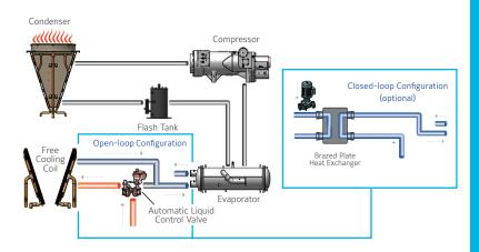
3 Free Cooling Mode At lower ambient temperatures, full cooling load can be most efficiently delivered by the free-cooling coils. Compressors are shut off and the VSD fans are modulated to meet the cooling setpoint.
